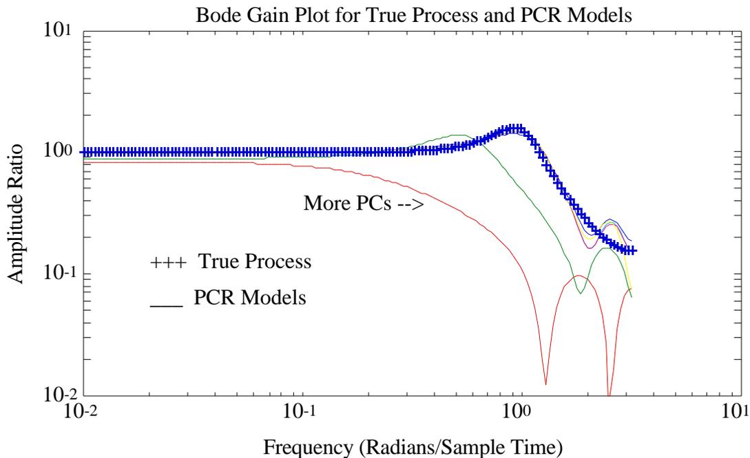
Figure 16. Bode Gain Plots of Process Model 7 and ARX Models Identified with PCR.
