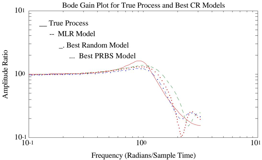
Figure 21. Bode Gain Plots for True Process and ARX Models Determined by CR and MLR.
