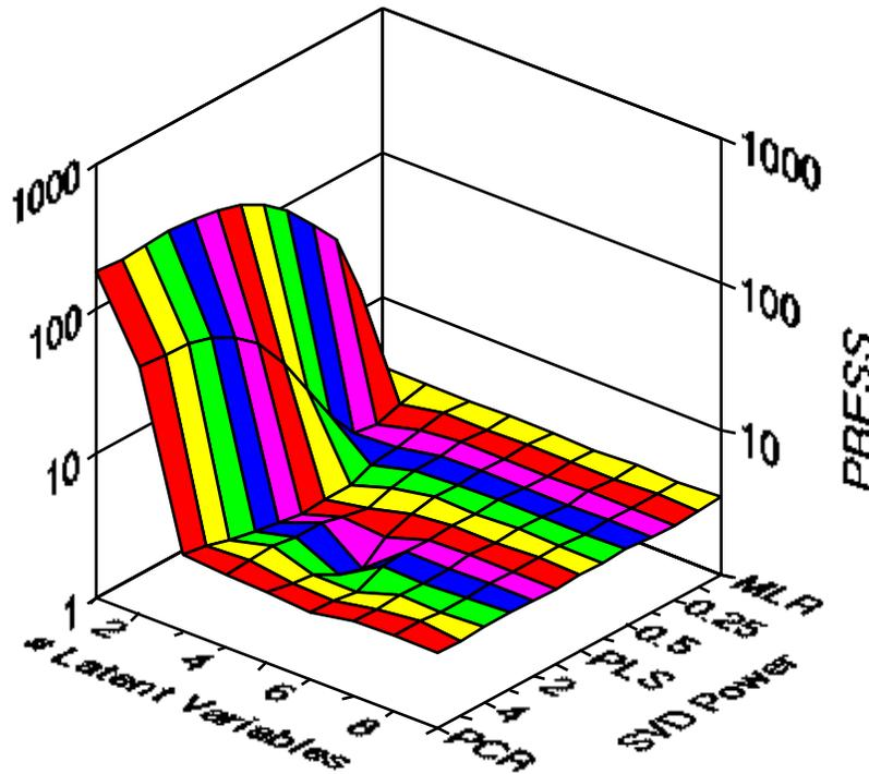
Figure 17. PRESS Surface for ARX Models Tested Against PRBS.
