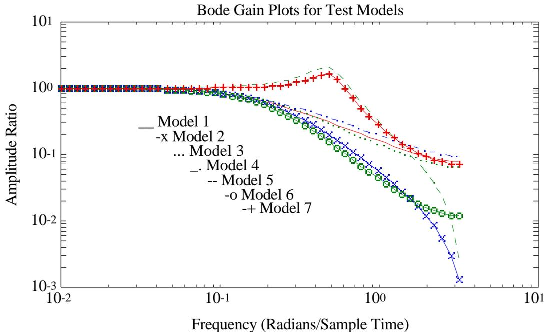
Figure 7. Bode Gain Magnitude Plots for the Seven Test Processes.
