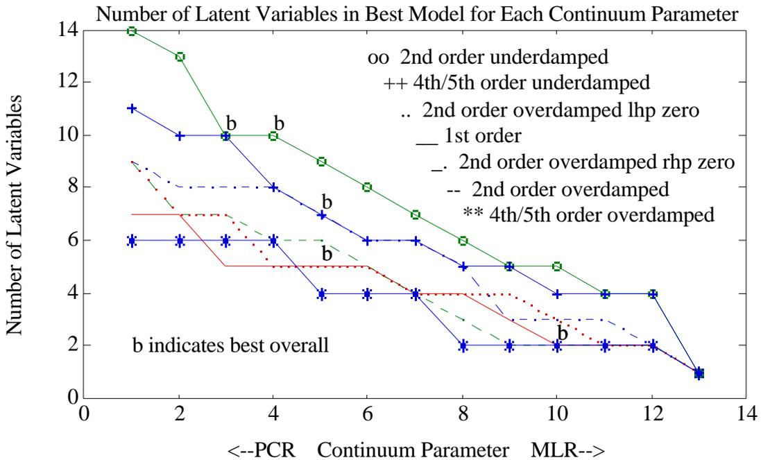
Figure 11. Effect of Process Dynamics on Number of Latent Variables in Best Model for Each Continuum Parameter
