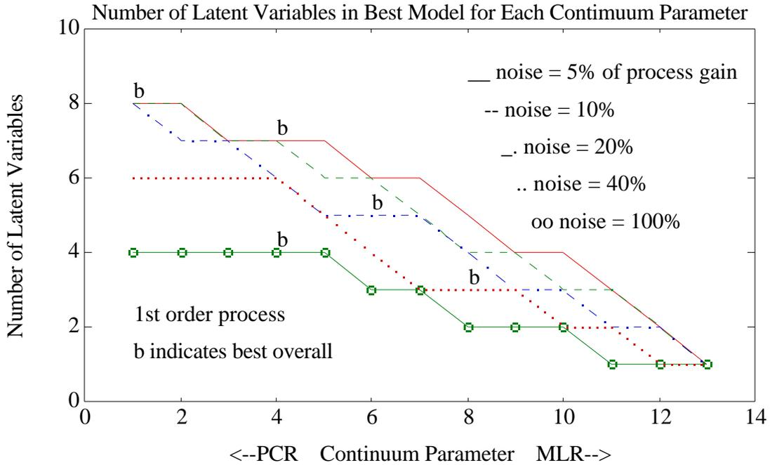
Figure 10. Effect of Process Noise Level on Number of Latent Variables in Best Model for Each Continuum Parameter
