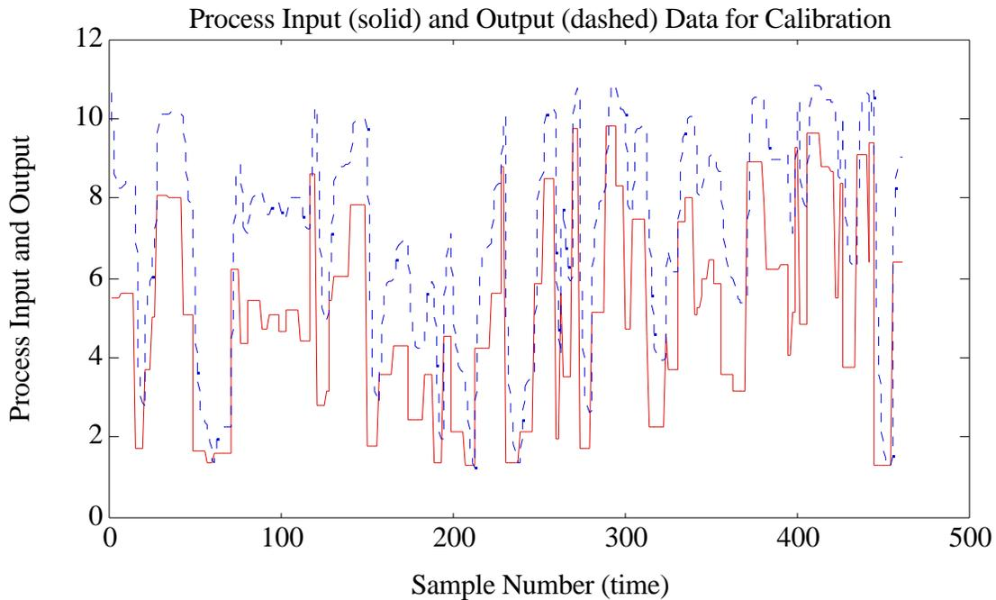
Figure 22. Non-Linear Tank Process Input/Output Data Used for Calibration
