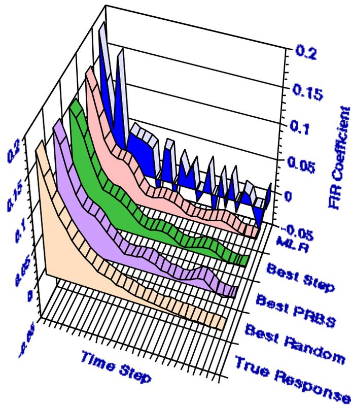
Figure 15. FIR Coefficients Identified from Second Order Over-Damped System with Noise = 20% of Process Gain
