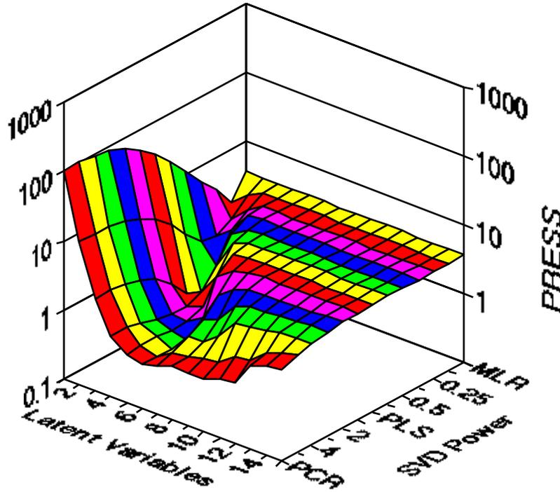
Figure 9. Continuum Regression PRESS Surface From Models of First Order Process with 40% Process Noise.
