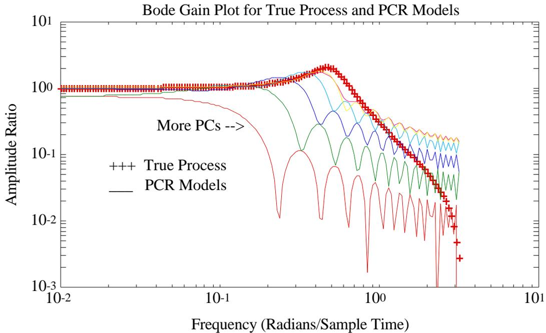
Figure 6. Bode Gain Magnitude for Second Order Process and PCR Models
