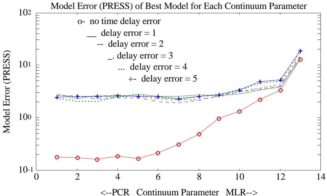
Figure 14. Model Errors for Correct and Incorrectly Estimated Time Delays.
