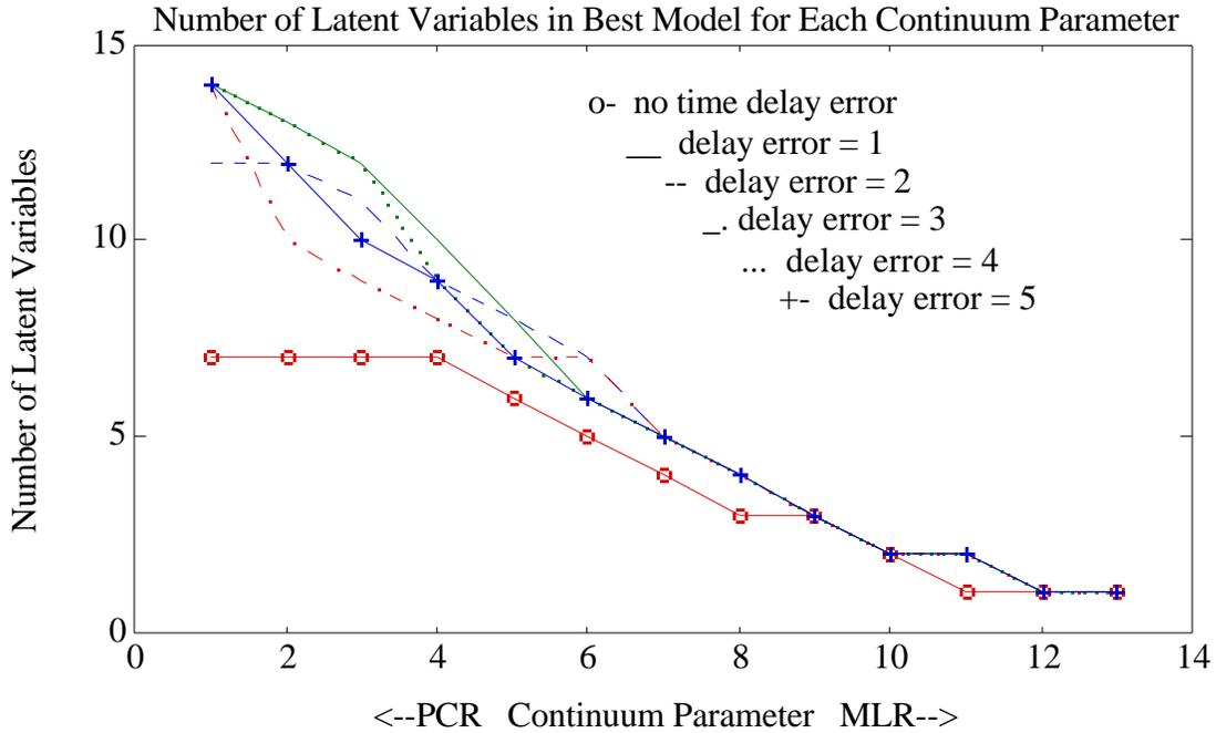
Figure 13. Effect of Mis-Estimated Time Delay on Number of Latent Variables in Best Model for Each Continuum Parameter
