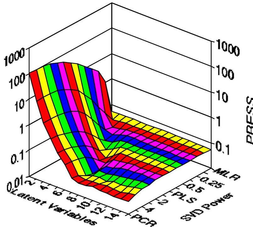
Figure 8. Continuum Regression PRESS Surface From Models of First Order Process with 5% Process Noise.
