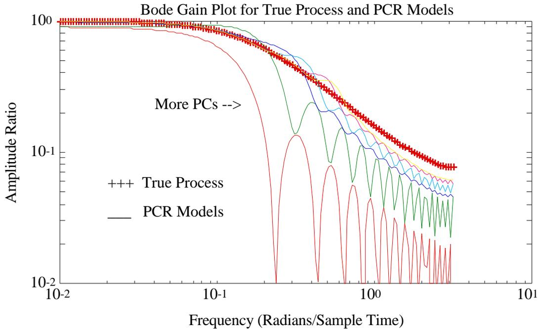
Figure 5. Bode Gain Magnitude Plot for First Order Process and PCR Models.
