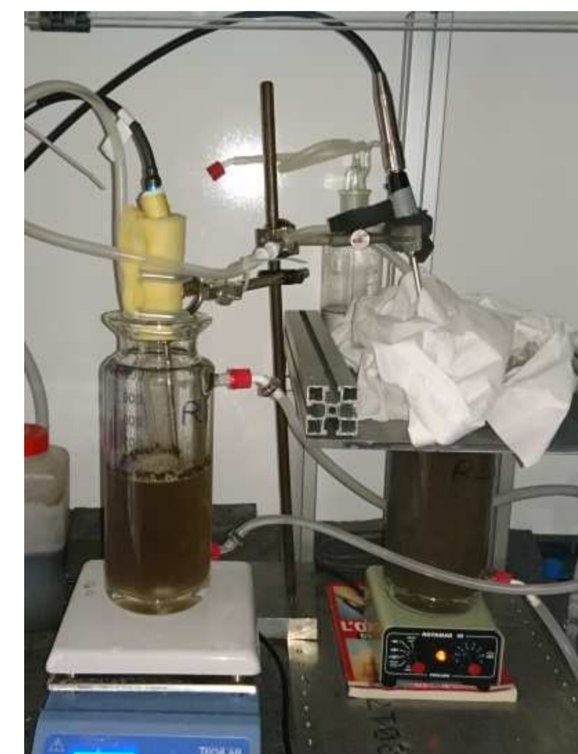
Raman immersion probes during the biodegradation test of a fluorinated ether
